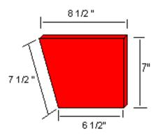
Next cut the front, back and bottom boards. The dimensions for the length should be the one determined by your windows. The width of the front board will be the total width of your board, 7 ½ (assuming you are using 1x8's). The back board is cut square 7 inches wide. The bottom board should be cut 5 inches wide with a 20 degree angle to make it meet the front board squarely on the front. (5 inches will be the short dimension).
