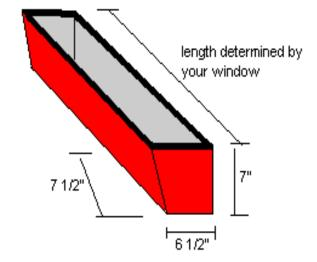
Pressure treated wood is hard to come by in all the sizes you need, though it is getting better. My boxes are built, to a degree based on the available lumber size. I have found pressure treated 1x8's, so 7 ½ inches has become my largest dimension. This keeps you from having to joint two boards together.
