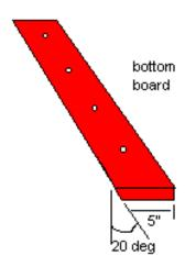
To assemble your box, use galvanized exterior wood screws and galvanized 6d finishing nails. The screws should be 1 ½ long. I always countersink the screws and cover them with elmer's wood filler. Drill ¼ inch holes, about an 1/8 in deep, 2 for each the front, bottom and back. Then drill the hole all the way through the end boards with a bit about the size of your screws threads.
