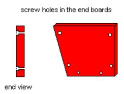
Now screw the end boards on to the front, back and bottom. The exterior screws shouldn't need a pilot hole in the front, back and bottom boards, however if they are hard going in, put a little soap on the threads to make them go in easier.
